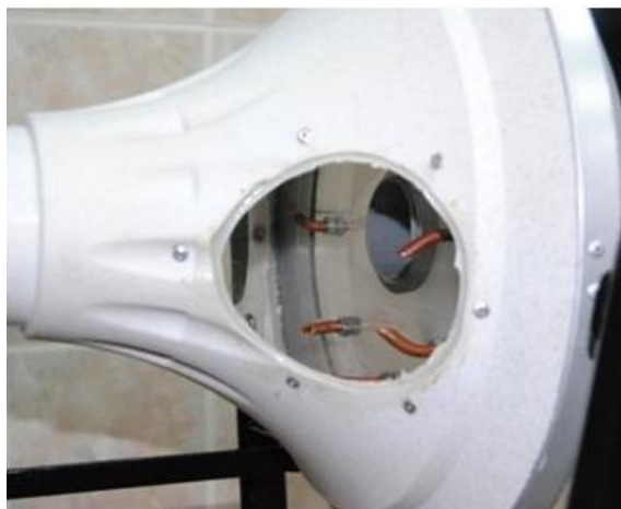
Fig. 3. Structurally and technologically improved mixing chamber in accordance with (Orekhova, et.al., 2018) (the mixing chamber is made with adjustable blower pipes)
