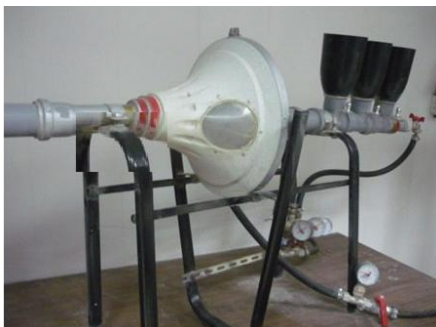
Fig. 1. Experimental sample of the basic design of a pneumatic mixer
